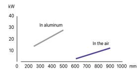
The power ratings range from 2 to 12kW in the air and from 14 to 27kW in aluminum at 700°C, corresponding to heating lengths from 250mm to 900mm.
