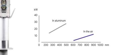
The power ratings range from 2 to 12kW in the air and from 14 to 27kW in aluminum at 700°C, corresponding to heating lengths from 250mm to 900mm.
