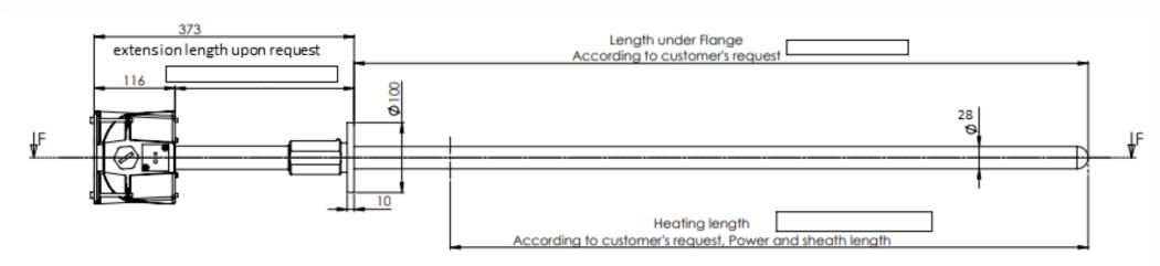
Different connectors & extension lengths available (cable gland or quick plug, upon request).
