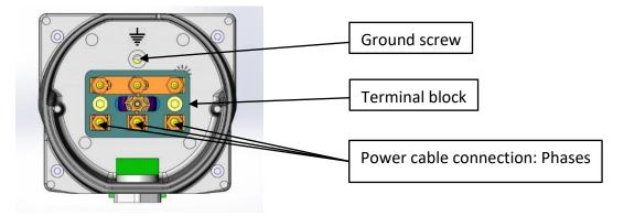
Remove the ground screw and connect the ground cable. Retighten the screw to a max. torque of 3 Nm.
