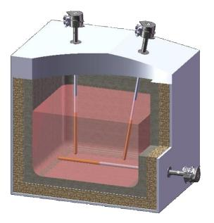
It is mandatory that the heating length stays totally immersed in the liquid metal while working.
