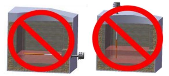
It is absolutely mandatory to avoid any contact with the furnace walls and with solid objects introduced into the bath (aluminium ingots, NC parts).
