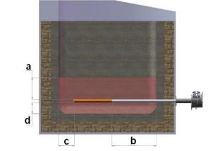
**a:** distance between the top of the heating length and the bath level.
