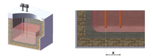
Centre-to-centre distance X minimum = 100 + immersion heater diameter.
