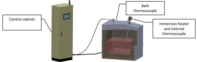
The control cabinet must be able to adjust the power of any immersion heater(s) installed in the furnace. The setpoint temperature is checked with the bath thermocouple. The power distributed to the immersion heaters is modulated, according to the value of this temperature.
